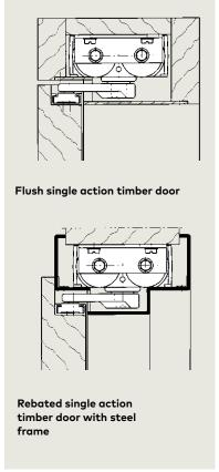
Detailed 1:1 scale installation drawings are available on request.
